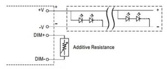
"DO NOT connect "DIM- to -V"
