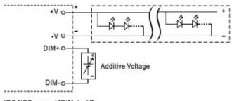
"DO NOT connect "DIM- to -V"
