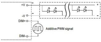
"DO NOT connect "DIM- to -V"
