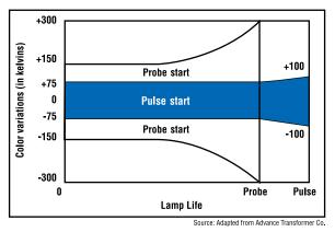
Pulse Start technology significantly reduces color shift providing consistent color over the life of the lamp.
