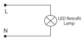
Easy to install - bypass ballast and provide voltage directly to lamp
