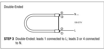
**CAUTION:** Use only non-shunted lampholders for Single-Ended wiring installations. Do not perform Single-Ended wiring installation of product in a fixture with shunted lampholders (found in all fixtures using instant start ballasts). If the existing lampholders are shunted, and Single-Ended wiring is desired, remove and replace them with non-shunted lampholders (or remove the external shunt if applicable). Make new connections directly to lampholder terminals as shown in Figure 1 below.
